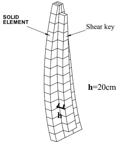
Fig.5 The key structure joint model with magnification of height of shear key
