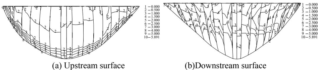
Fig.3 Envelop of Maximum principle tensile stresses on the dam surface (FJB, Unit:MPa)
