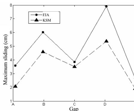
Fig.10 The maximum sliding of the joints at the top of arch dam
