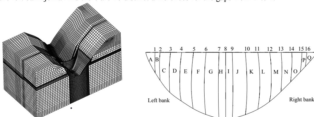
Fig.1 The finite element discretization of arch dam-foundation and the setup of contraction joints
