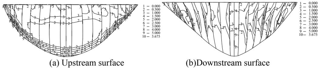
Fig.2 Envelop of Maximum principle tensile stresses on the dam surface (FJA, Unit:MPa)
