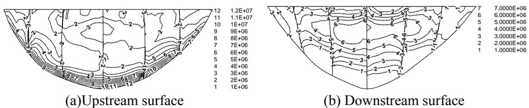
Fig.8 Maximum values of maximum principle tensile stresses on the upstream(KSM, Unit:Pa)
