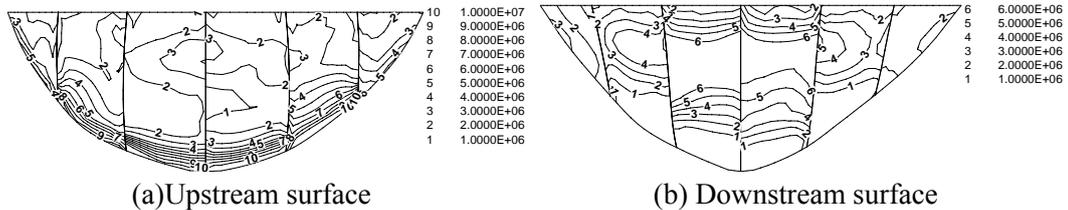
Fig.6 Maximum values of maximum principle tensile stresses on the upstream(FJA, Unit: Pa)
