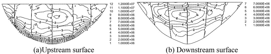
Fig.7 Maximum values of maximum principle tensile stresses on the upstream (FJB, , Unit: Pa)
