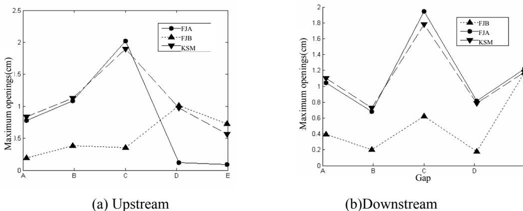
Fig.9 The maximum openings of the joints at the top of arch dam
