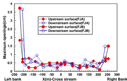
Fig.4 The maximum openings of the joints
