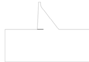
b) Propagation of crack profile at the heel of the dam at t=4.228 sec
