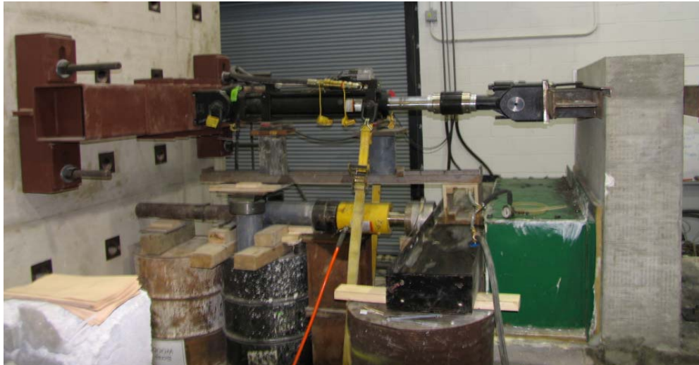
Figure 1 Test set-up for a wall-foundation specimen
