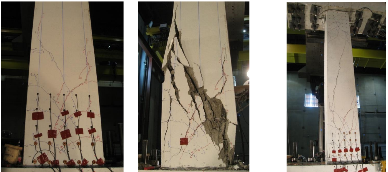
Figure 3. (a) Specimen 1 prior to axial failure (b) Specimen 1 after axial failure (c) Specimen 2 after axial failure
