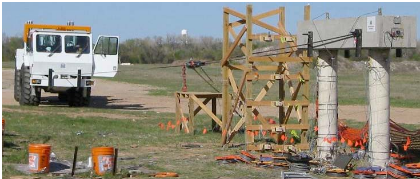
Figure 4 T-Rex preparing to pull on Bent#1 (credit: S.L. Wood)
