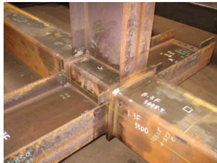
Figure 3 Details of base and beam-column connections (NRIESDP, 2007)
