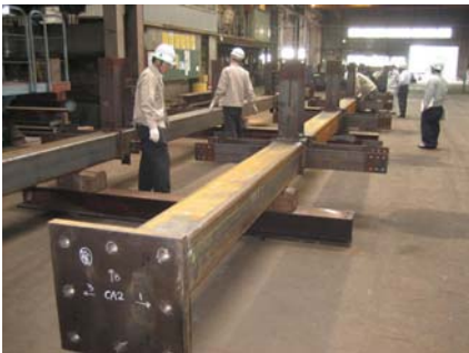
Figure 3 Details of base and beam-column connections (NRIESDP, 2007)
