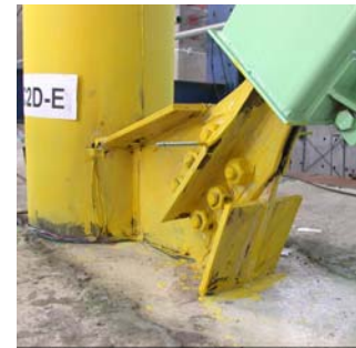
Figure 5 Added stiffeners at the free edges of the gusset at the brace to column joint before Phase-2 tests
