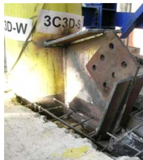
Figure 5 Added stiffeners at the free edges of the gusset at the brace to column joint before Phase-2 tests
