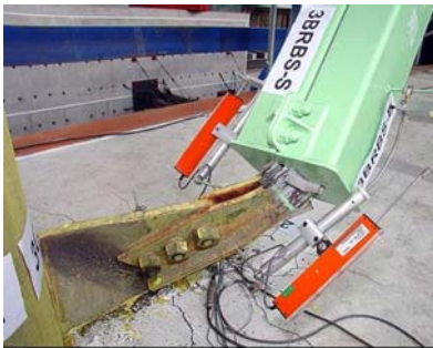
Figure 4 Buckling of the gusset at the brace to column joint after Phase-1 tests
