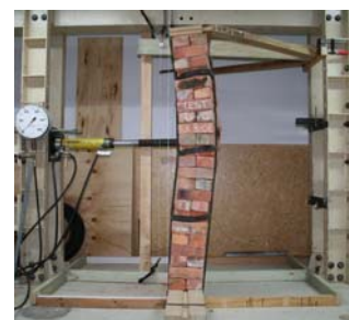
Figure 11 Out-of-plane load transferred vertically.
