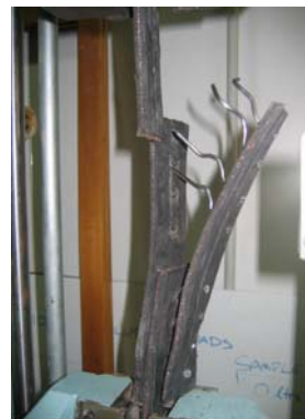
Figure 6 A failed connection where the originally bent nails have pulled-through.
