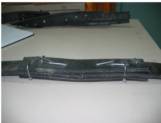
Figure 5 A completed nailed joint showing the bent nails that prevent premature nail pull-through.
