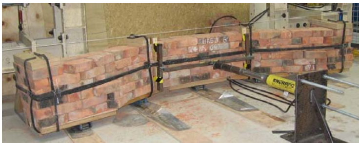
Figure 10 The out-of-plane test set-up with the wall pushed towards its supports.
