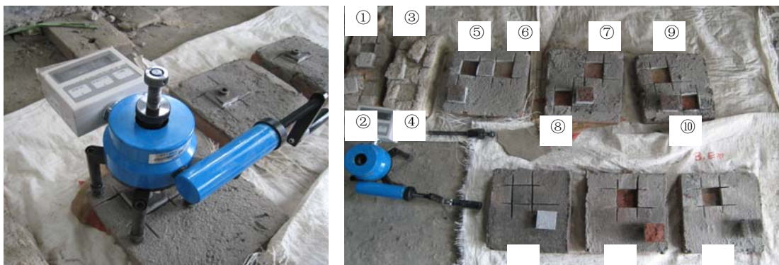
Photo.2 Tensile strength test by BRI method
