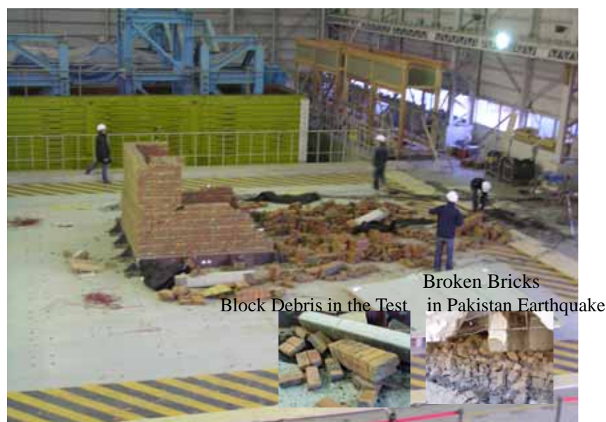
Figure 12. Collapsed Test House
