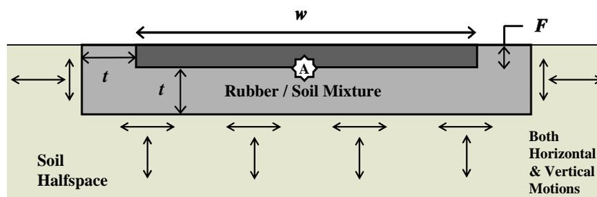
Figure 3 Simplified model for finite element analysis using *QUAD4M*.
