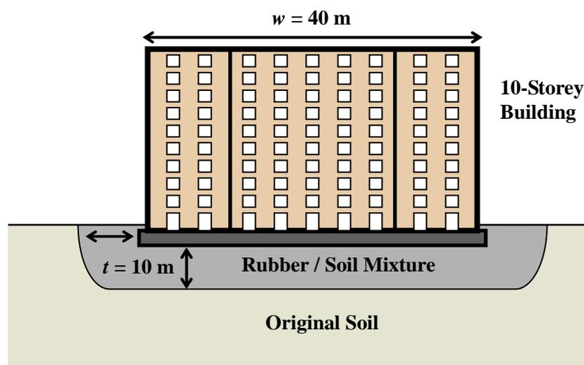
Figure 1 Seismic isolation by a layer of rubber-soil mixture (RSM) (Tsang, 2008).
