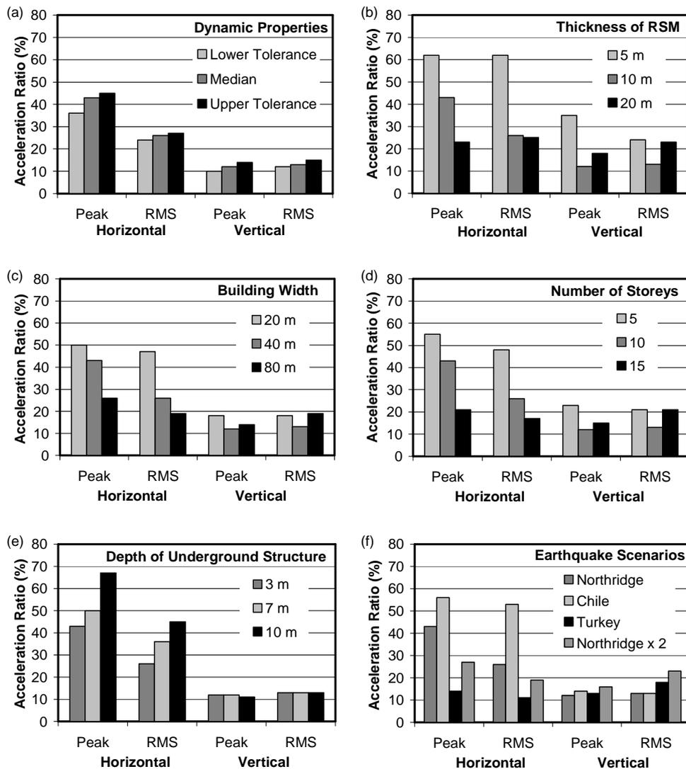
Figure 5 Comparison of the acceleration ratio, with respect to different (a) dynamic properties of RSM; (b) thicknesses of RSM; (c) building widths; (d) number of storeys; (e) depths of underground structure; and (f) earthquake scenarios (Tsang, 2008). *Notes:* Only one input parameter was varied in each case, while all other input parameters were held constant at the default values specified for the **Reference** scenario.
