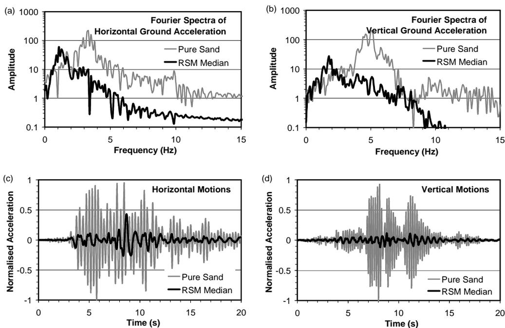
Figure 4 The *Fourier* amplitude spectra (*FAS*) of the (a) horizontal and (b) vertical ground accelerations; and the corresponding normalized (c) horizontal and (d) vertical ground acceleration time histories for the **Reference** scenario (Tsang, 2008). *Notes*: In each figure, the scenarios of placing RSM and pure sand were plotted. Each time history was normalized by the respective maximum absolute ground acceleration of the scenario with pure sand.
