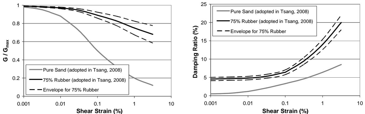
Figure 2 (a) Shear modulus degradation curves and (b) damping curves (Tsang, 2008).
