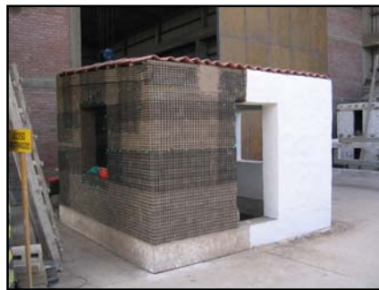
Figure 2. Model reinforced with geogrid, half plastered
