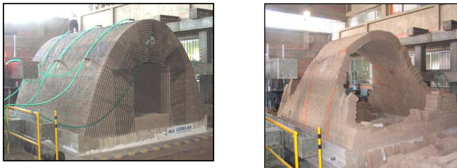
Figure 4. Reinforced vault and non reinforced vault after test.
