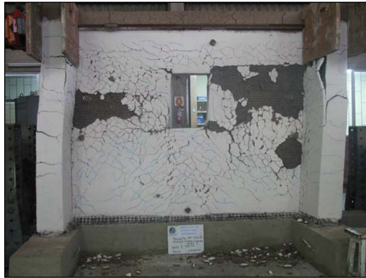
Figure 5. Cyclic shear test on reinforced adobe wall.
