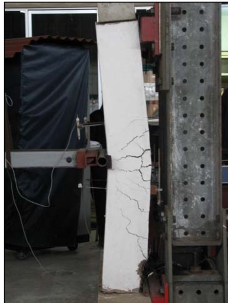
Figure 7. Out of plane bending test on reinforced adobe wall.
