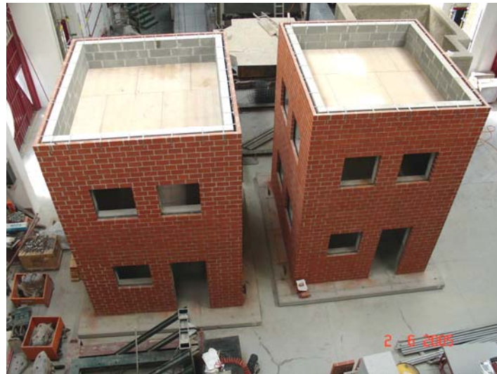
Figure 2 – The two models at the end of construction, Model 1 on the right and Model 2 (reinforced house) on the left
