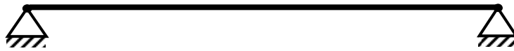
Figure 4: An axially restrained beam with rectangular cross-section of span L = 6000 mm; depth d = 100 mm; width w = 50 mm; Young's modulus E = 2.05 \times 10^5 N/mm 2 ; yield stress \sigma_y = 300 N/mm 2 ; and coefficient of thermal expansion \alpha = 12 \times 10^{-6} /° C.
