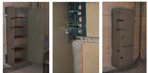
Figure.11. Installation of the cabinet for testing
