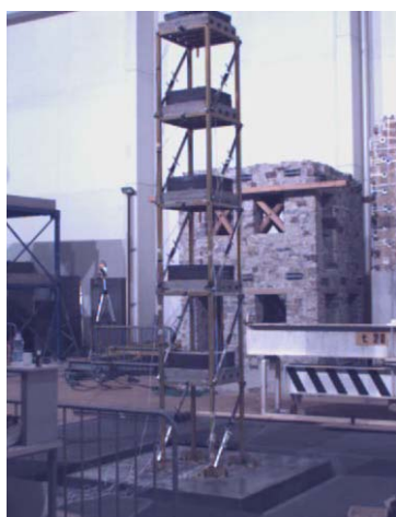
Figure 8 Earthquake response of steel 5-storey frame (left) and response history of roof floor (right)
