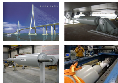
Fig.4 Sutong Bridge and dampers
