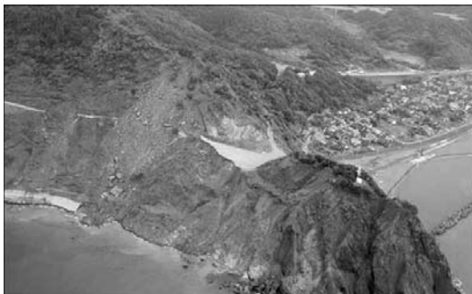
Photo 15 Slope failures along the multiple dip surfaces at Hijirigahana (Photo:By Pasco Co.)
