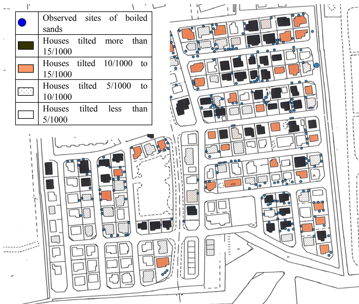
Figure 3 Distribution of the rank for angle of inclination of houses in Abehikona housing development
