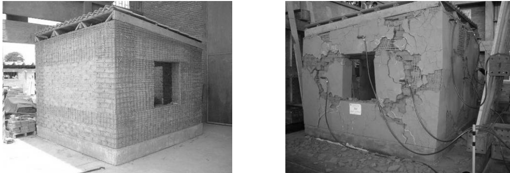
Figure 10 Adobe model reinforced with plastic mesh
