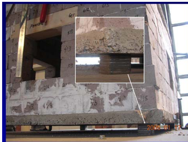
Figure16 Load-displacement curve of STP Figure17 Specimen of seismic isolation device of STP
