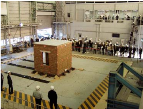
Figure10 Shaking table experiment on December 27, 2007
