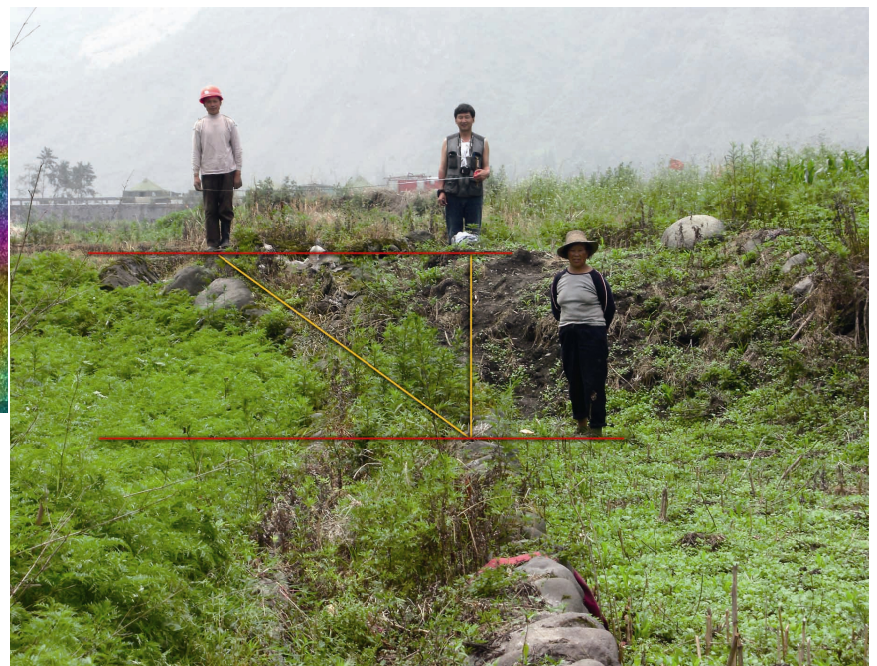
Figure 6 The N20W left-lateral strike-slip fault with dip-slip cut and uplifted irrigation canal with the maximum displacements of 2.8m in horizontal, and 1.5m in vertical(point B, left), in X(Xiaoyudong, left top), Pengzhou City. The length of the NW surface fault was identified over 2 km on both riversides, strath terrace. It broken down the Xiaoyudong bridge (Bridge), cut throughout the cone and vegetable farmlands, and destroyed the buildings and roads. By SAR interferogram, the NW left-lateral fault with about 10km length between LMS faults ① and ②, and ~4 km width. See text in detail.
