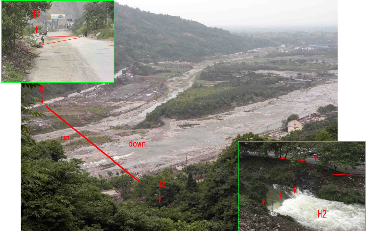
Figure 3 Looking northeast along the N40E-thrust fault with the maximum displacements of 1.5m in vertical, in Hanwang, Mianzhu City (Figure 1, Table 2.1). The 2km length of the fault was traced on riverbed, both riversides, strath terrace, and until mountain sides H1 and H2.
