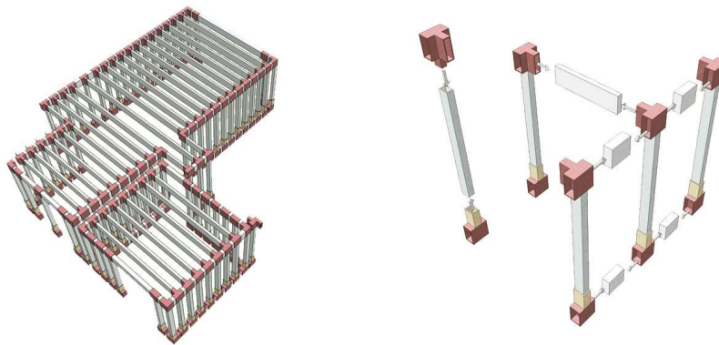
Figure 11 & 12 – Partial perspectives of the bare bone framing and assembly of the add-on FRP components
