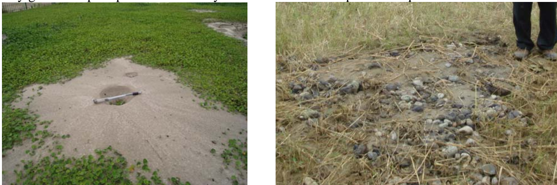
Figure 9 Sand boils and gravelly sand ejected (Photo by Z. Cao)
