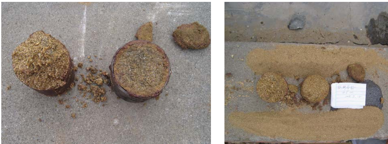
Figure 13 Sandy soil sampled compared with the sands ejected (Photo by W. Wang)
