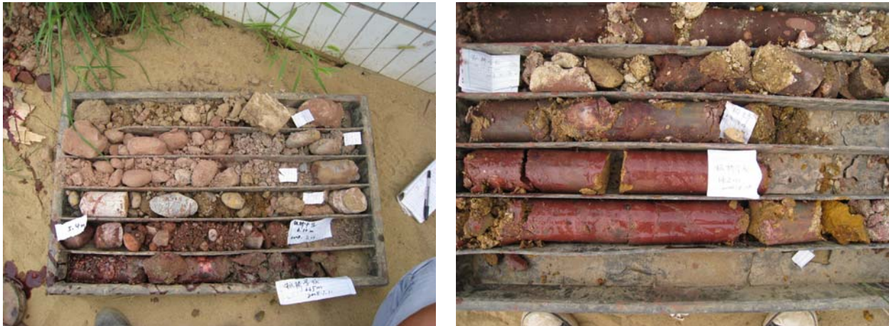
Figure 12 Soils sampled from the borehole (left picture shows soils of 0 to 6.65m and right picture shows soils of 6.65m to 15.4m ) (Photo by W. Wang)
