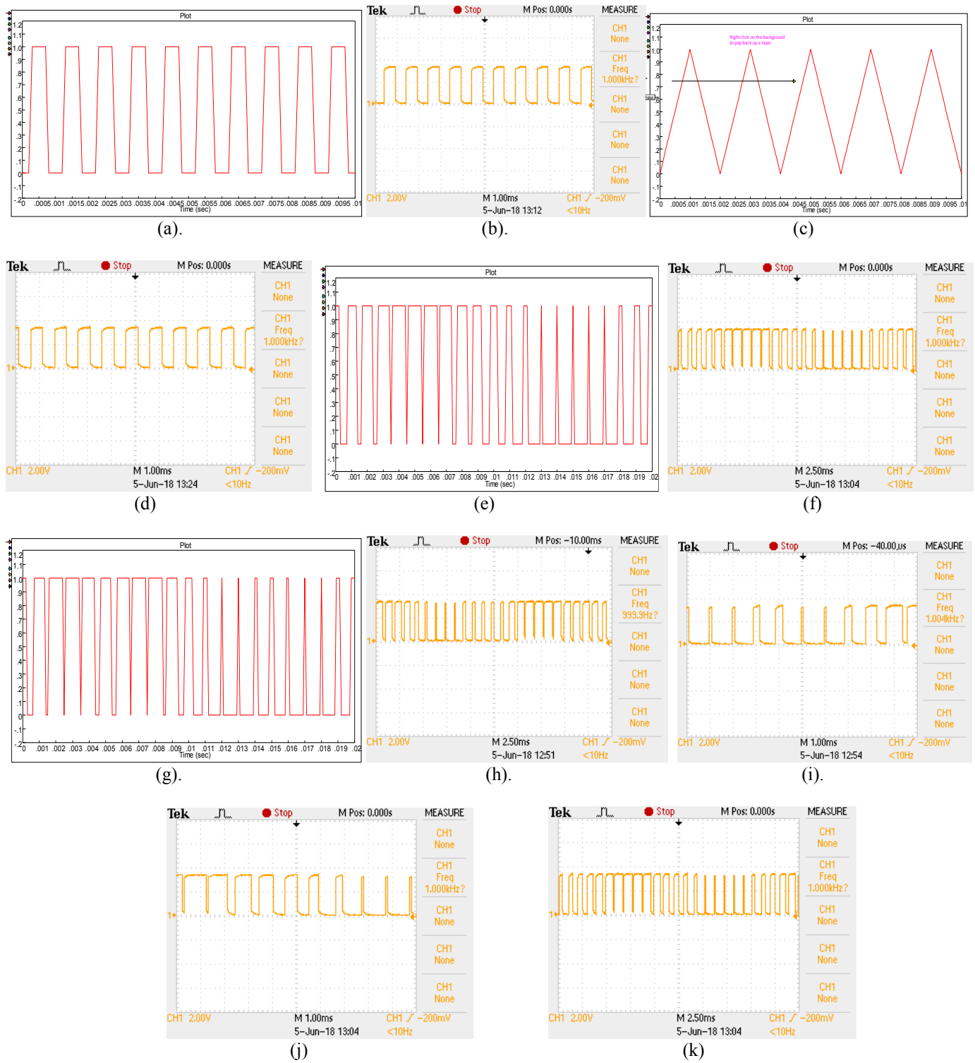
Fig. 6. (a) Fixed duty constant frequency PWM signal generation (simulated) (b) Fixed duty constant frequency PWM signal generation (practical) (c) Triangular carrier frequency of 500 Hz (simulated) (d) Fixed duty 1Khz frequency PWM signal generation from half carrier frequency i.e. 500Hz. (e) Sin-Triangle PWM generation (Simulated-M-0.8) (f) Sin-Triangle PWM of 1kHz switching frequency (Practical-M-0.8) (g) Space Vector PWM generation for 1kHz switching frequency (Simulated-M-0.8) (h) Space Vector PWM generation for 1kHz switching frequency (Practical-M-0.8). (i) Small increase in duty ratio near zero crossing for space vector PWM (j) Duty ratio changes sinusoidally near zero crossing for Sin-Triangle PWM. (k) Sin-Triangle PWM of 1 kHz switching frequency (practical-M-0.75).
