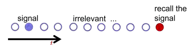
Figure 4.10: A schematic view of the long short term memory. Selective memory is being maintained for long term, is allowed to be modified, and is available for use with short-term memory to produce responses. This is unfolding of recursiveness.
