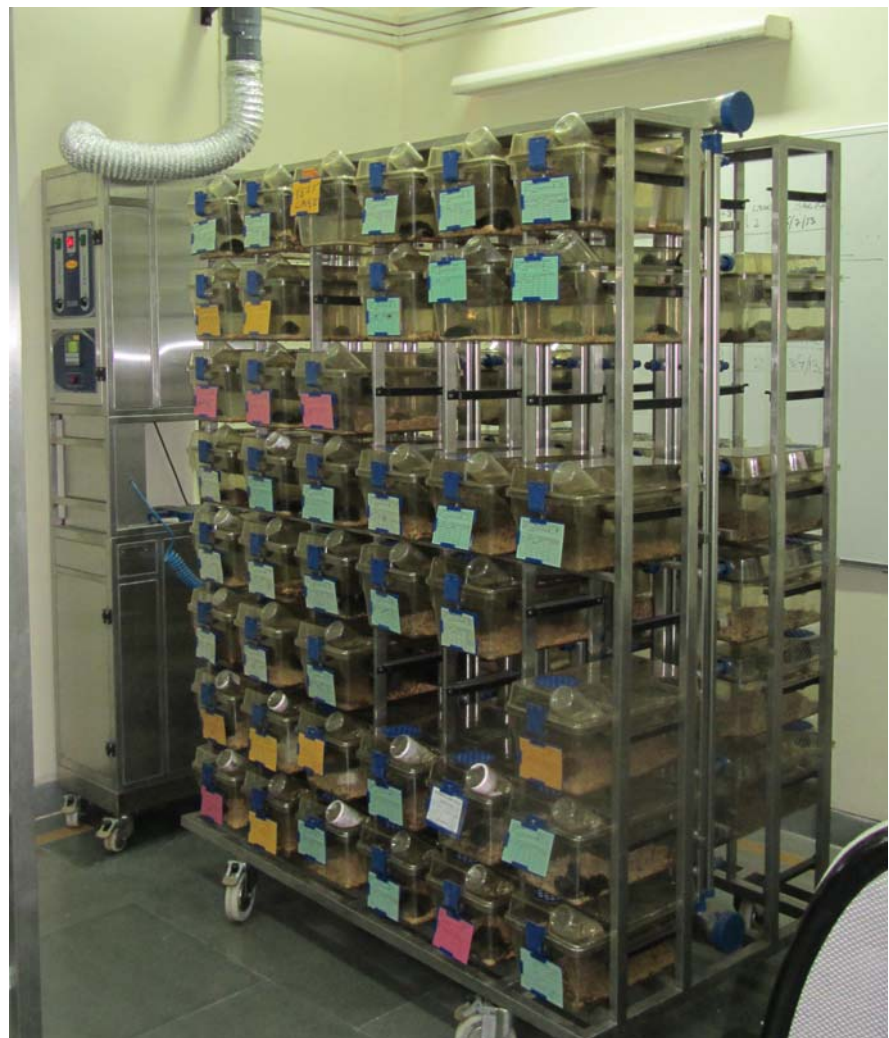
Photograph showing the individually ventilated cage system and the ventilator installed in the BSBE laboratory to house transgenic mice
