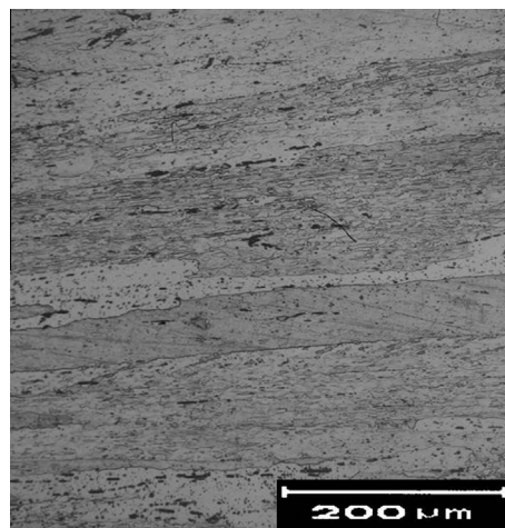
Fig. 1. Initial microstructure of the material used in the present study. The material is in as forged condition and has elongated grains in the direction of perpendicular to the direction of forging.
